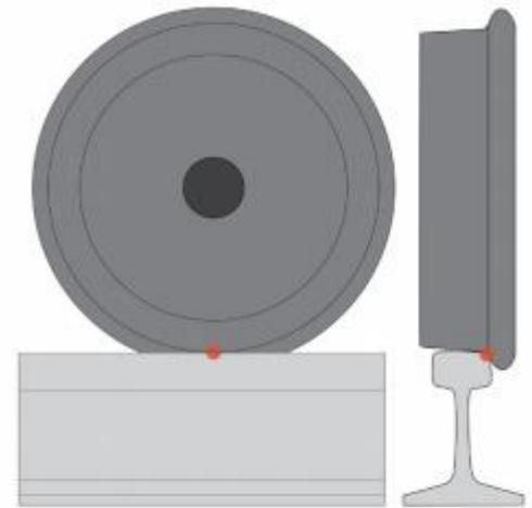
1. The electrical contact between wheels & rail is on the inside rail head and quite small.
